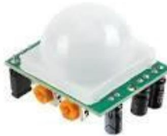
Gambar 2.3 Sensor *Passive Infra Red*
